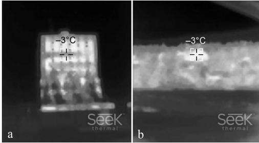
**FIGURE 5.** a. Thermal image of the south face of the Alberta Grain Terminal in Edmonton, Alberta, Canada, on a sunny day (9 February 2019), with a surface temperature of  $-3^{\circ}\text{C}$  and ambient temperature of  $-26^{\circ}\text{C}$ . b. Thermal image of a bare cliff face on the North Saskatchewan River (12 February 2019) on a sunny day with a surface temperature of  $-3^{\circ}\text{C}$  and ambient temperature of  $-21^{\circ}\text{C}$ .
