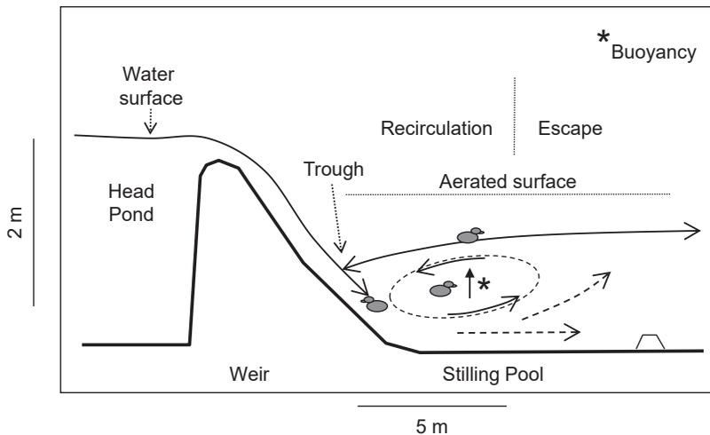
**FIGURE 2.** A cross-section of the Calgary weir and hydraulic recirculation zone with scaling based on Makuk (1988) and Golder (2002). The positions of the submerged ducklings are based on flume simulations with objects of similar buoyancy and observed emergence patterns. Note the exaggerated vertical scale.
