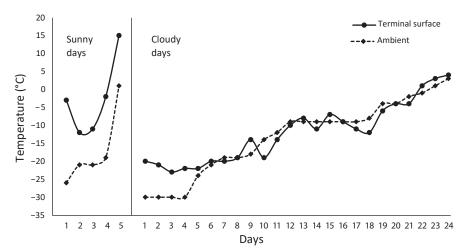
FIGURE 4. Surface and ambient temperature of the south face of the Alberta Grain Terminal in Edmonton, Alberta, Canada, on sunny (n = 5) and cloudy (n = 24) days in winter, 2019.
